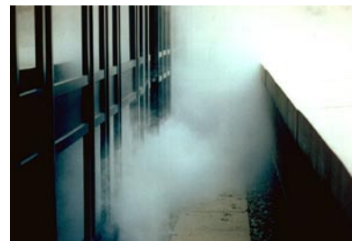
Undergoing a smoke test under pressurisation exposes this building's frightening lack of airtightness! Source: A. Leaman & W. Bordass, www.usable-buildings.co.uk
